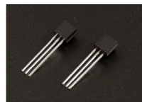
Strictly selected pair-matched special FET (common to 700T and 700S)
